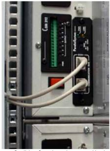
Parallel configuration and programmable relay contacts board
